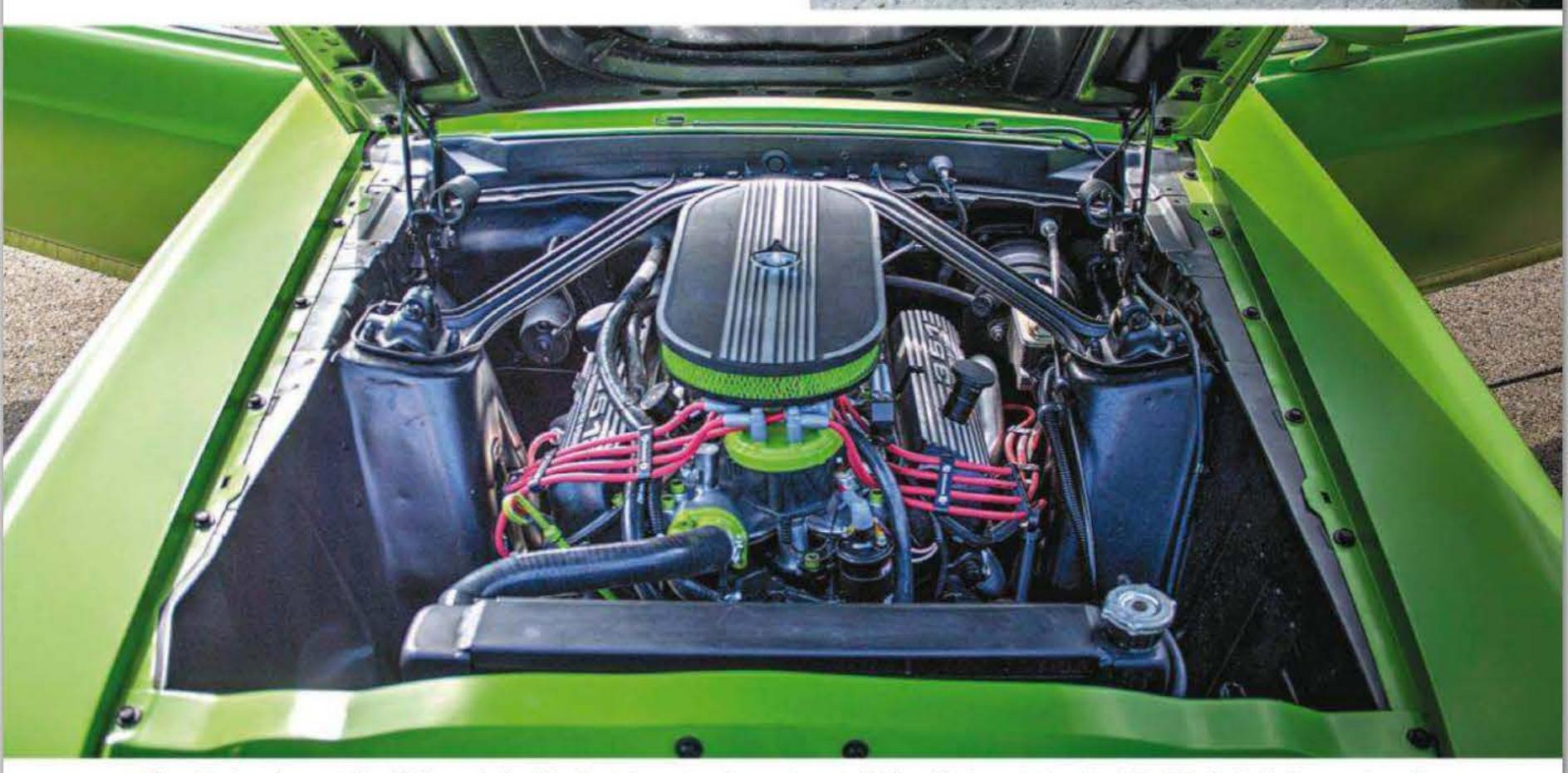
The original, numbers-matching 351W was rebuilt with beefy rotating parts and a ceramic-coated Edelbrock Performer intake with a Holley 750-cfm Double Pumper, a Comp Cams 270H hydraulic cam, a MSD Pro Billet distributor, a Blaster 2 coil, and MSD wires. Hedman ceramic-coated headers and dual 21/4-inch exhaust with Flowmaster mufflers make up the exhaust. The fuel system is all hard lined. There's a 100-amp alternator, aluminum radiator, and a Hitachi high-torque starter.
